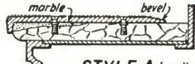
STYLE A - long lip for worn wood or marble treads maximum depth of lip 2" from underside of tread.
